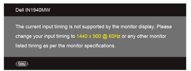
This means that the monitor cannot synchronize with the signal that it is receiving from the computer. See <u>Monitor Specifications</u> for the Horizontal and Vertical frequency ranges addressable by this monitor. Recommended mode is 1440 x 900.
