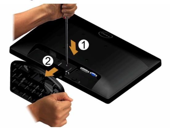
To remove the stand assembly from the monitor:
