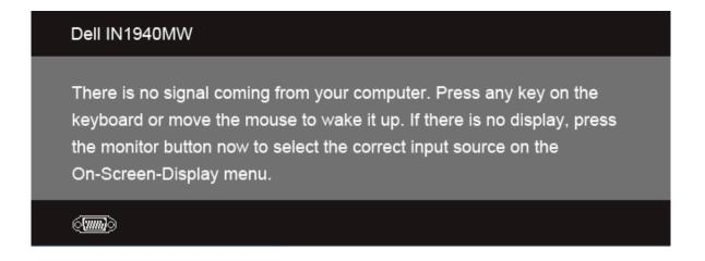
If either VGA or DVI-D input is selected and both VGA and DVI-D cables are not connected, a floating dialog box as shown below appears.
